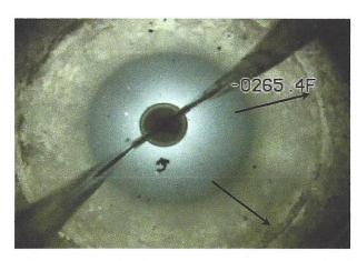
Photo 026 Top of fill. Weight dropped off at 273.7' indicating TD
